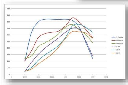
The EcoBoost V-6 does reach its maximum torque sooner and has a broader torque range than the other engines, but that's how turbos work. There's a reason it's so popular in Ford trucks.
