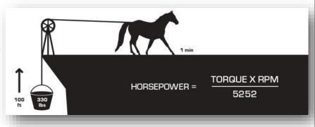
same time. Or, 1,000 pounds of coal could be raised 33 feet in one minute. These are all calculations for one horsepower or 33,000 lb-ft of torque per minute.
