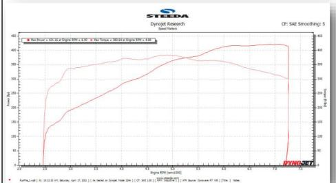
than the specs provided by Ford. This is normal when measuring output from the wheels versus the crankshaft (which is what manufacturers do). Another term for this difference is *drivetrain loss*.
