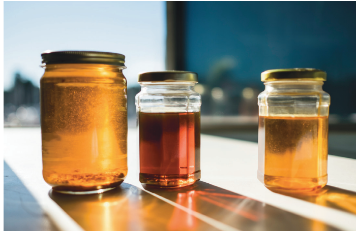
THESE THREE JARS OF DIESEL OIL, WHICH HOLM DERIVED FROM PLASTIC DEBRIS FROM THREE DIFFERENT SOURCES, SHOW HOW IMPURITIES IN THE PLASTIC CAN FOUL THE FUEL AND COMPROMISE USABILITY.
