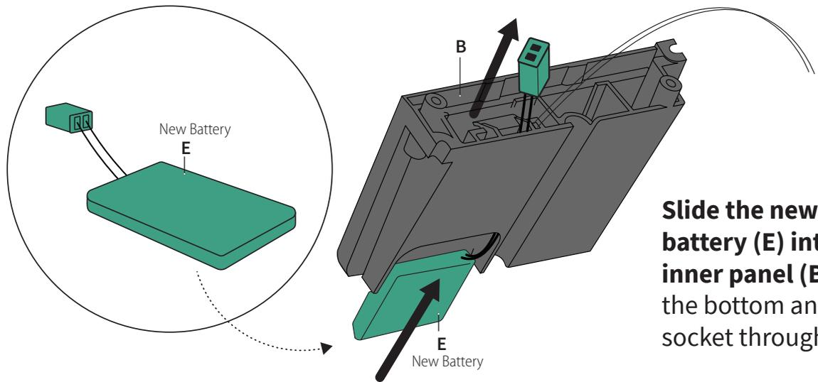
**Slide the new Li-ion battery (E) into the inner panel (B) from the bottom and pull socket through the top.**
