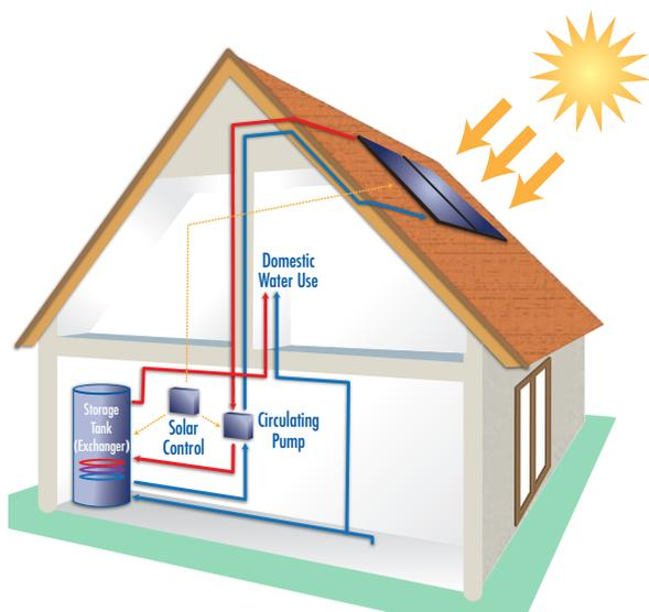
Figure 2. Residential solar water heating system schematic
